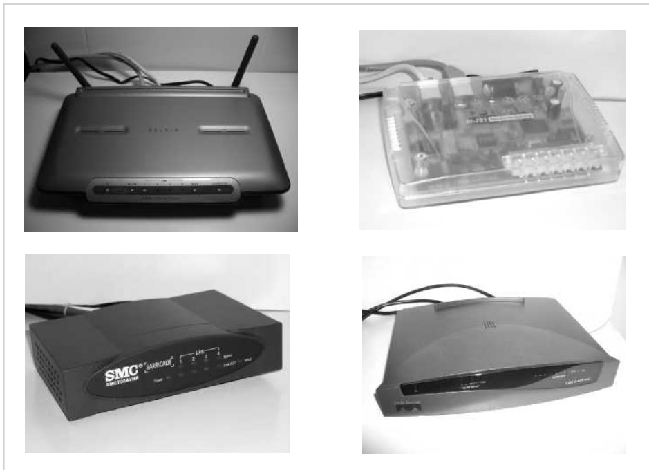
Figure 6-7 SOHO Firewall Devices
